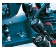
operator to engage free-fall whenever desired without removing his hands from the control levers.
