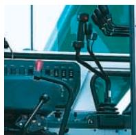
Function lock lever prevents accidental operation when the operator enters or leaves the cab.
