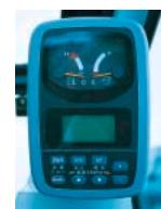
The easy-to-read LCD multi-display provides current status information on such functions as engine rpm, maintenance and on-board trouble-shooting, providing the operator with an ongoing real-time assessment of the machine's conditions at a glance.
