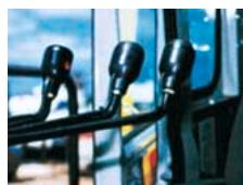
Full-hydraulic technology delivers quick, efficient operation with excellent precision. Pilot pressure-assisted control allows you to control the speed and power of each function in proportion to lever movement.
