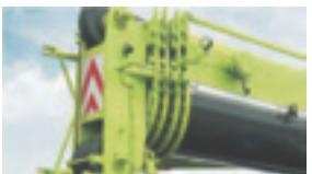
The ZRT850 features a 5-section, U-shaped ,47m telescopic boom.It's telescoping system consists of a two-stage hydraulic cylinder with a rope extension mechanism.
